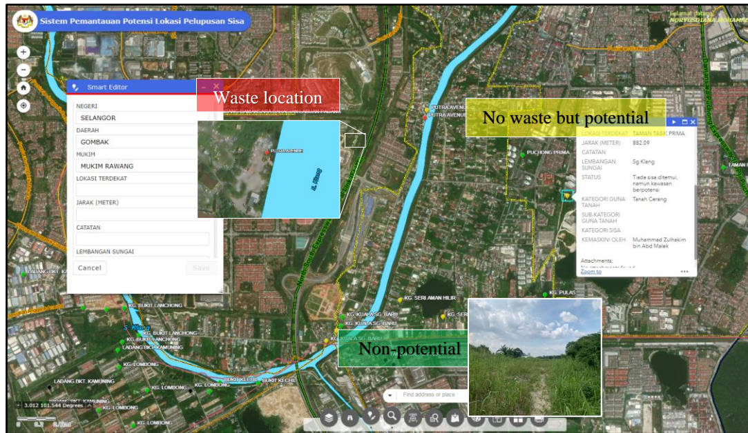
Figure 10. Smart editor allows users to classify the waste potential hotspot status into three (3) options - a) waste location; b) no waste but potential area; or c) non-potential
